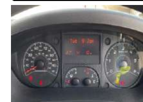
Dials for RPM, fuel and engine temperature - needles have been removed as this information is not required on e-Relay
